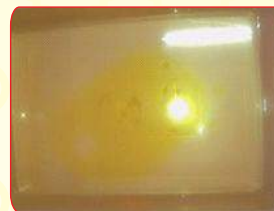
Testing the Bio mat Tray with 1 litre water and 50 ml oil
